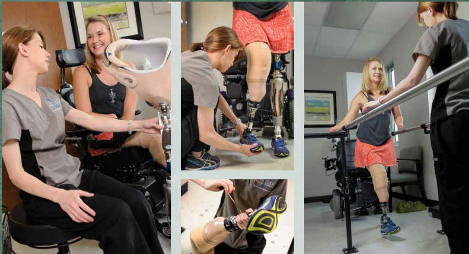
Prosthetist Rachel Schmidt of ProCare Prosthetics adjusts Copeland's leg, which has a microprocessor in the knee with angle and load sensors that analyze her gait while she's walking as well as how much weight she puts on her toe and heel. Alignments are made by linking the knee through Bluetooth to the computer, but Schmidt can also make manual adjustments.
